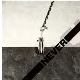
Photograph E (Typical) Excessive side-loading.
