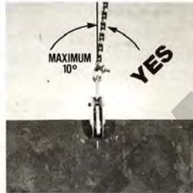
Photograph D (Typical) Maximum allowable side-loading.
