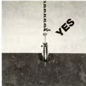
Photograph C (Typical) Sling directly above and in line with lifting shackle.
