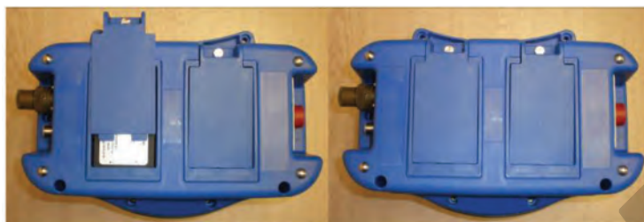
Fig. 7: Installation of Battery Cover – XLTX
