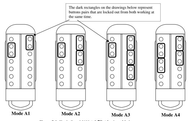
Figure 7-8. Single-Speed 9100 telePilot Lockout Modes.
