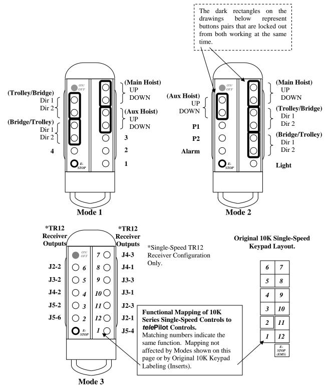
Figure 7-7. Single-Speed 10K telePilot Modes.
