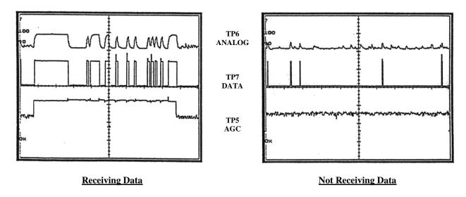
Figure 9-2. Receiver Scope Wave Forms.
