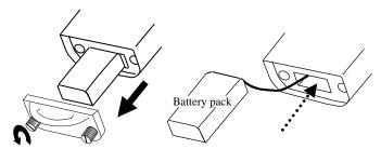
Figure 7-9. telePilot Infrared Port Access.
