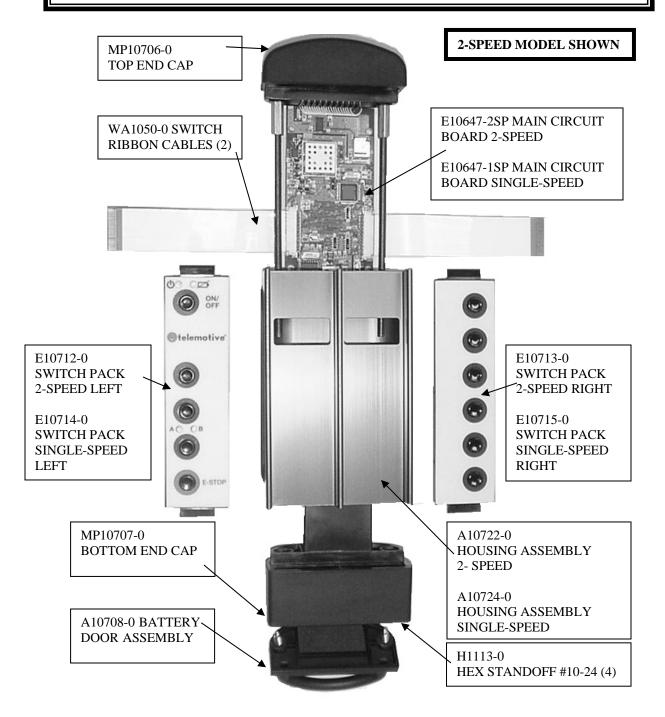
Figure 10-1. telePilot Exploded View.
