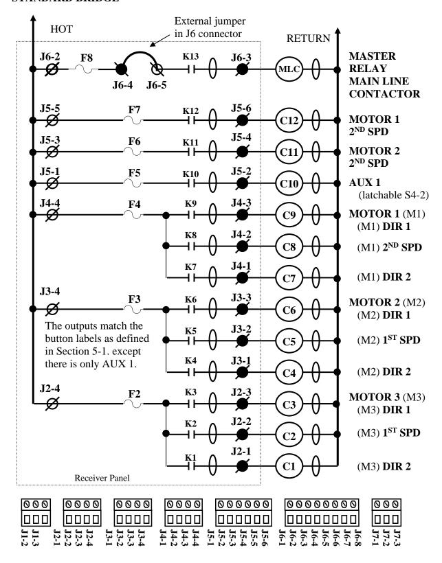
TABLE 2(E) TR12 2-SPEED PROGRAMMING DIAGRAM. P&H: 2-SPEED, 2-WINDINGS for HOIST and TROLLEY; STANDARD BRIDGE
