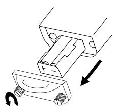
Figure 5-3. telePilot Battery Replacement.
