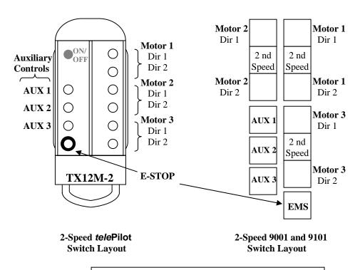
Figure 7-9. Functional Mapping of 9001 and 9101 Series 2-Speed Controls to *tele*Pilot Controls.
