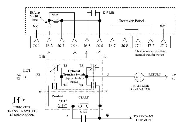
Figure 6-2. External Transfer Switch Wiring
