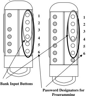
Figure 5-2. Bank and Password Input Buttons.
