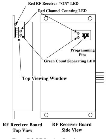
Figure 7-2. RF Receiver Board.
