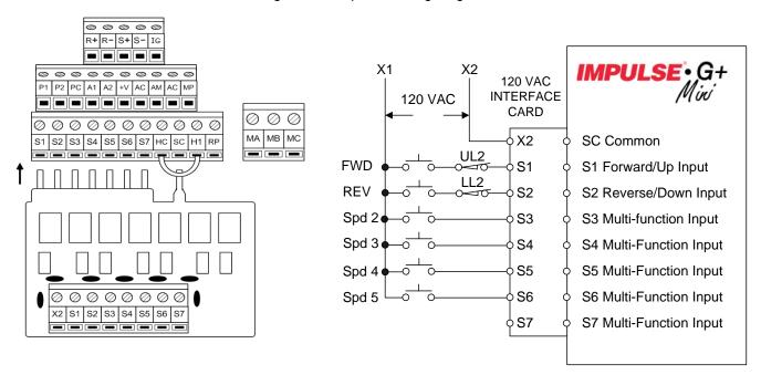
Figure 1. Typical 120 VAC Interface Card Wiring
