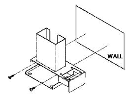
Figure 6: Wall mounted housing
