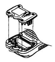
Figure 2: Inserting the Battery Pack
