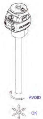
Diagram 5H3. Proper use of Force Sensing Handle grip.
