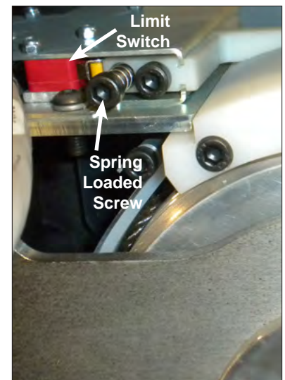
Diagram O. Locate socket head cap screw head and fully push it in until it can not move anymore.
