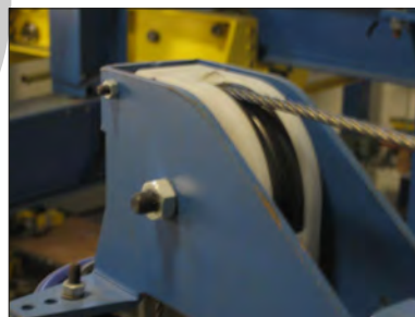
Diagram V. Pulley block at end of arm.
