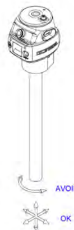
Diagram 6E3. Proper use of Force Sensing Handle grip.
