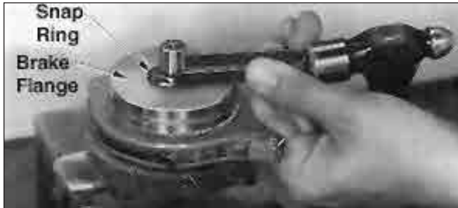
Figure 5-6. Remove Snap Ring From Load Brake Shaft
