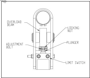
Figure 7-3a. Over-Capacity Limit Switch ("B" & "C" Frames)
