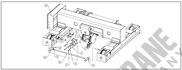
Figure 9-3a. Traverse Drive Component ("B" Frame Shown).
