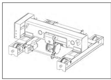
Figure 5-9. Traverse Drive Arrangement ("B" Frame shown above)
