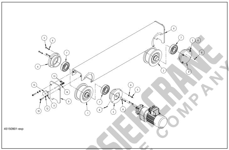
Figure 9-3d. Common Traverse Drive Components ("D" Frame)
