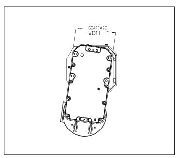
Figure 4-2. Gearcase Width Illustration
