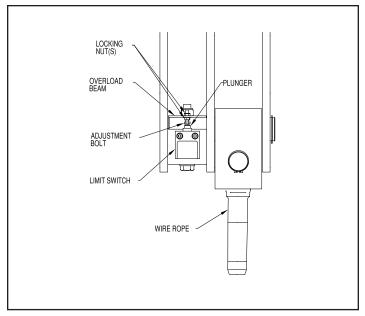
Figure 7-3b. Over-Capacity Limit Switch ("D" Frame)
