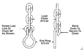
G. Assemble the end ring (673-53) to the free (loose) end of chain by rotating the last link 1/4 turn and passing the ends of the ring thru the link as shown below. Hammer or squeeze the ends of the ring together to secure it to the chain.
