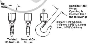
Any hook that is twisted or has excessive throat opening indicates abuse or overloading of the unit. Other load-sustaining components of the hoist should be inspected for damage.
