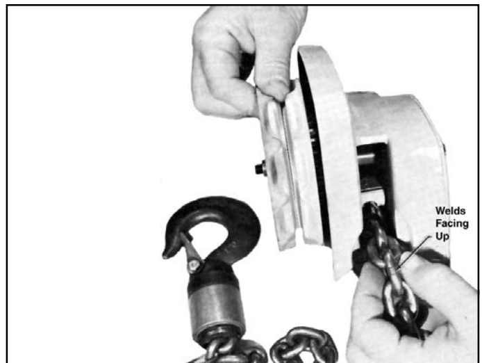
Figure 7-8. Installing Load Chain
