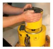
Remove motor bolts and pull motor away from gear case as shown in illustration.
