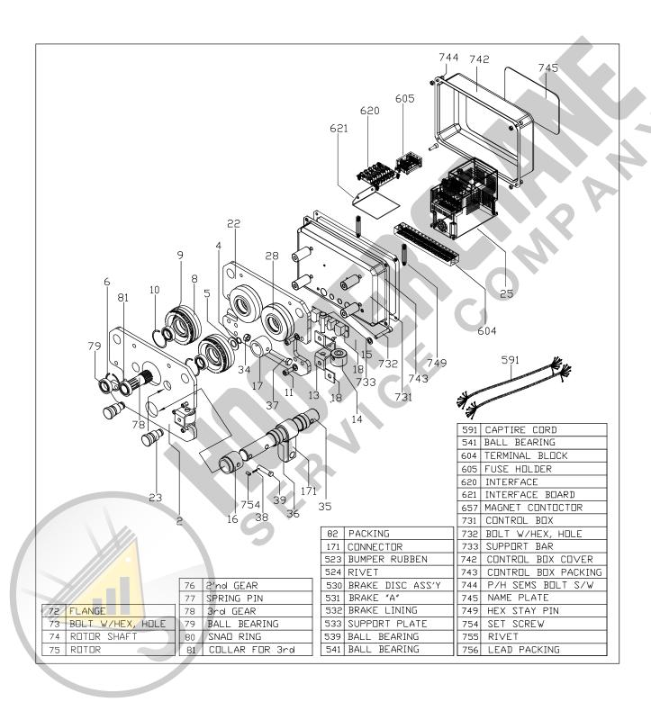
Except for inverter hoist assembly (no.23), inverter hoist interface (no.620,621), inverter trolley assembly (no.25), inverter interface (no.604,620,621,604), inverter hoist push button (no.19), all other parts are same as illustrated in ACCOLIFT® Electric Chain Hoist Manual 71575-06.
